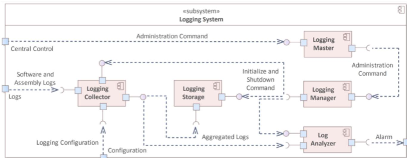
Fig. 1: Logical view of LOUD. Log sources are Alma Common Software (ACS) components, OPC UA servers and low-level software.
