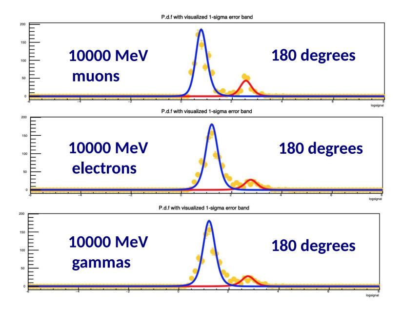
**Summary** : Full detailed GEANT4 simulations of a water Cherenkov detector were used to obtain a parametrization of the signal response. This parameterization will generate approximate signals which match the signals generated by the full detector simulation. In this way we can build a fast simulator of the detector.
