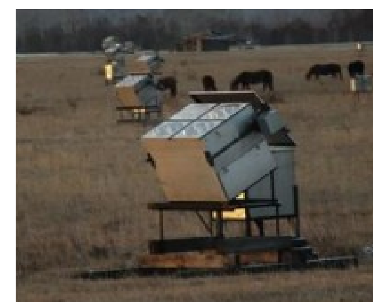
TAIGA-HiSCORE Integrating Air Cherenkov timing array – 120 stations
