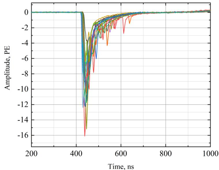
Typical pulse waveforms of muon event and other events
