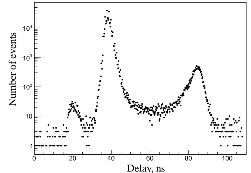
The SPE pulse waveforms, SPE and TTS distributions with a PMT gain of  $\sim 10^7$  and an amplifier gain of 10.
