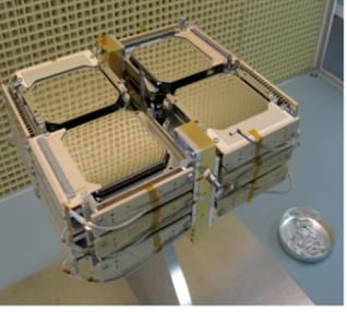
Fig. 1: COSI's detector volume comprised of 12 high-purity germanium semiconductor detectors (8 x 8 x 1.5 cm<sup>3</sup>, 2-mm strip pitch, energy resolution of 0.24% at 1.84 MeV)
