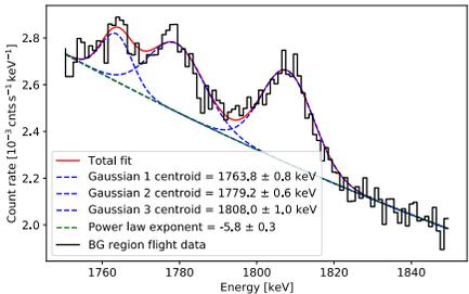
Gaussian shape parameters (Fig. 6) are included in a fit of the BG model, defined as the BG flight spectrum (Fig. 4) normalized to its mean.
