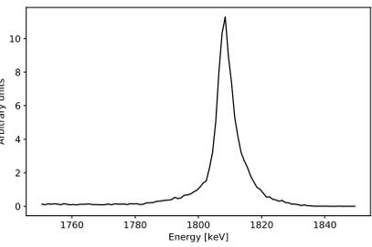
Fig. 6: BG model shape parameters: Power law + 3 Gaussians fit to all data in the background region
