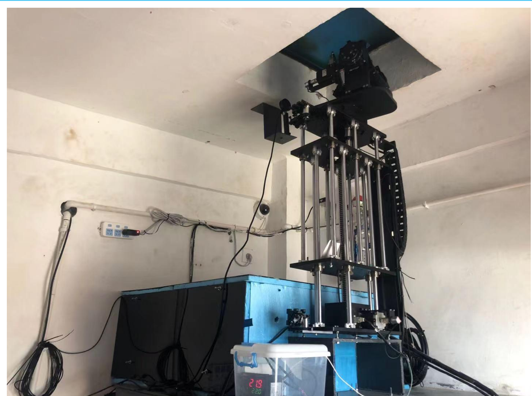
Figure 2: The schematic diagram of YAG Lidar inside the site, the black tank is the thermotank, YAG Laser and thermotank is located on an optic platform, the HiRoP is in the middle of the picture, mirrors and energy detector is coupled on the HiRoP.
