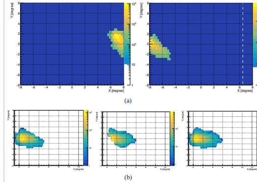
Figure 3: (a): The image of Cerenkov photons detected by T1 (left) and T2 (right) of WFCTA; (b): The image of the same event calculated for the virtual telescope, which points to the direction of the primary particle. Left: T1, middle: T2, right: T1 and T2 combined.
