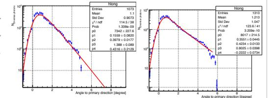
Figure 4: The distribution of  $dN/d\theta$  for the two events of cosmic ray data, red line is the fitted function of equation 1. Left: the event fully detected by single telescope; right: the event detected by two telescopes, and the images are combined together.
