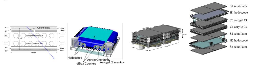
Figure 2: Left to right: TIGER stack, TIGER technical model, one of two SuperTIGER modules, and SuperTIGER module expanded view.
