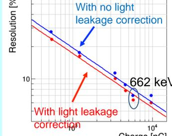
The energy resolution is roughly proportional to  $Q^{-1/2}$  (Q:charge), which follows statistical distribution of photo-electrons.
