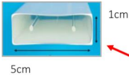
Extruded Scintillator bars with 2 holes
