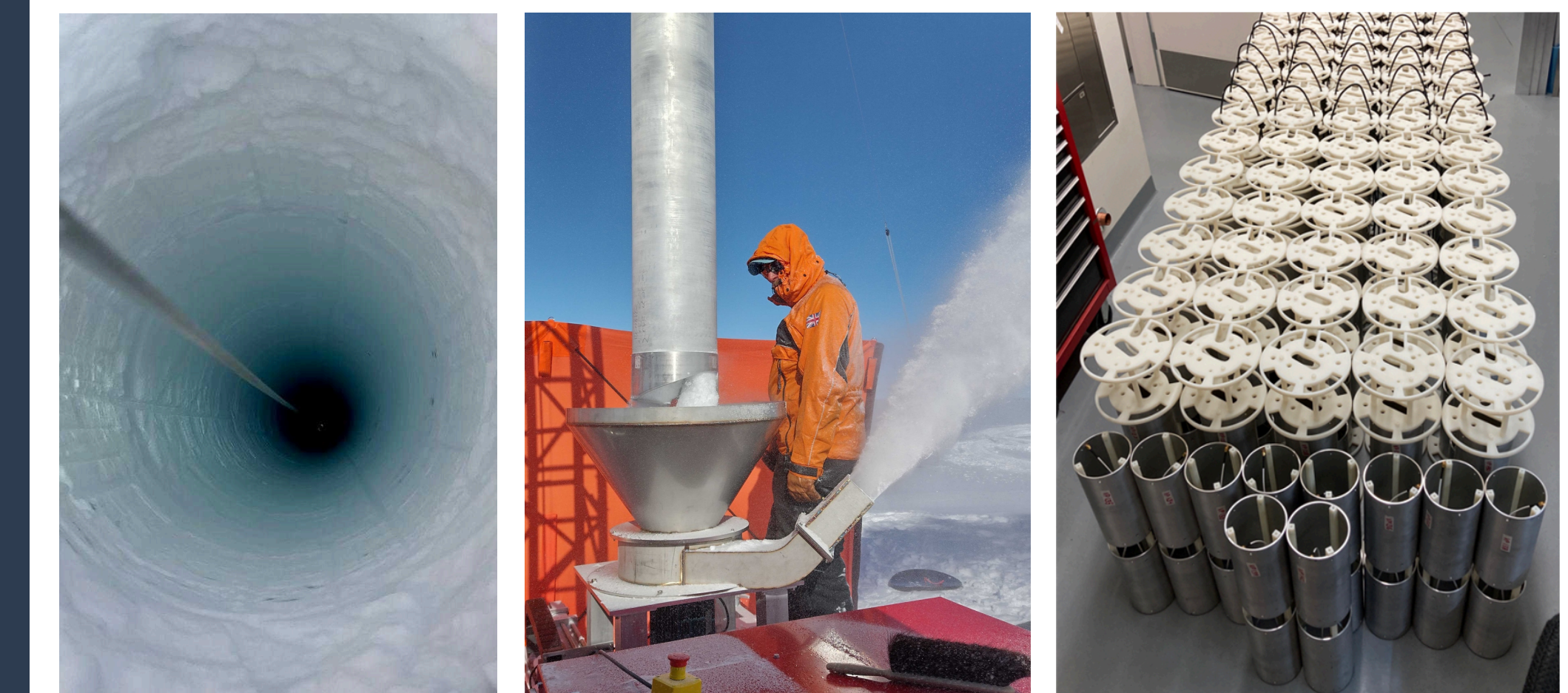
Fig 6: Top: DAQ box assembly line Left: Completed borehole. Middle: Ice drill ejecting chips Right: All assembled vertically polarized antennas
