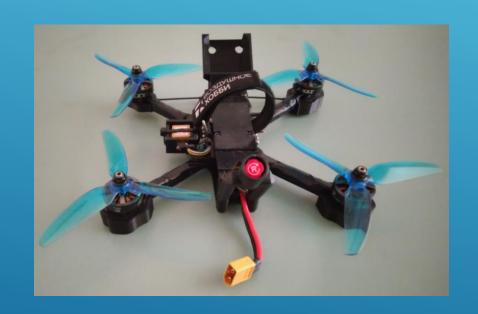
The drone can reach easily 500 m hight above EAS Cherenkov array and eleviate up to 300 g loading weight. The light source with its power supply and triggering pulse generator weighs well below 100 g. The pulse generator is based on Arduino Nano v3 plate with 8-bit microcontroller AVR ATmega328P (Atmel).
