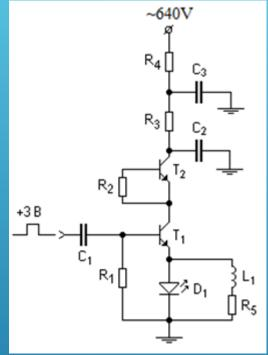
To get high light yield of the light source staying still in a few nanoseconds time domain the LED is driven by specially designed driver (Fig. 1) using a pair of avalanche transistors ZTX415 switched consecutively
