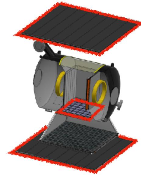
**Three layers of 1 cm thickness fast plastic scintillator, 2.3m top to bottom**
