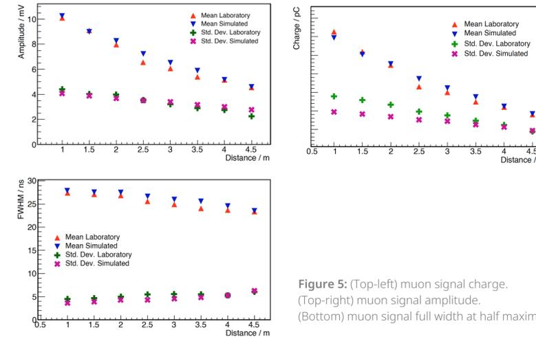
Figure 5: (Top-left) muon signal charge. (Top-right) muon signal amplitude. (Bottom) muon signal full width at half maximum.
