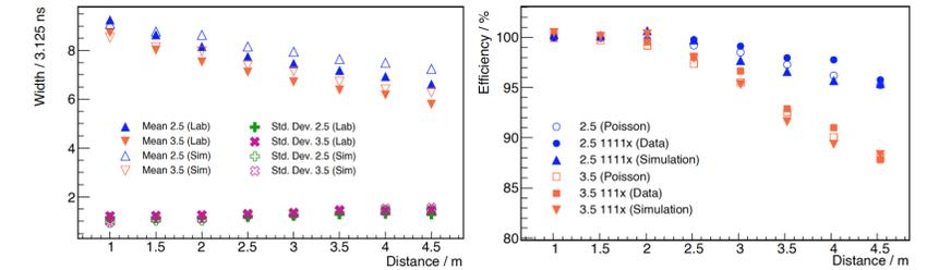
Figure 6: muon signal width (left) and muon detection efficiency (right).
