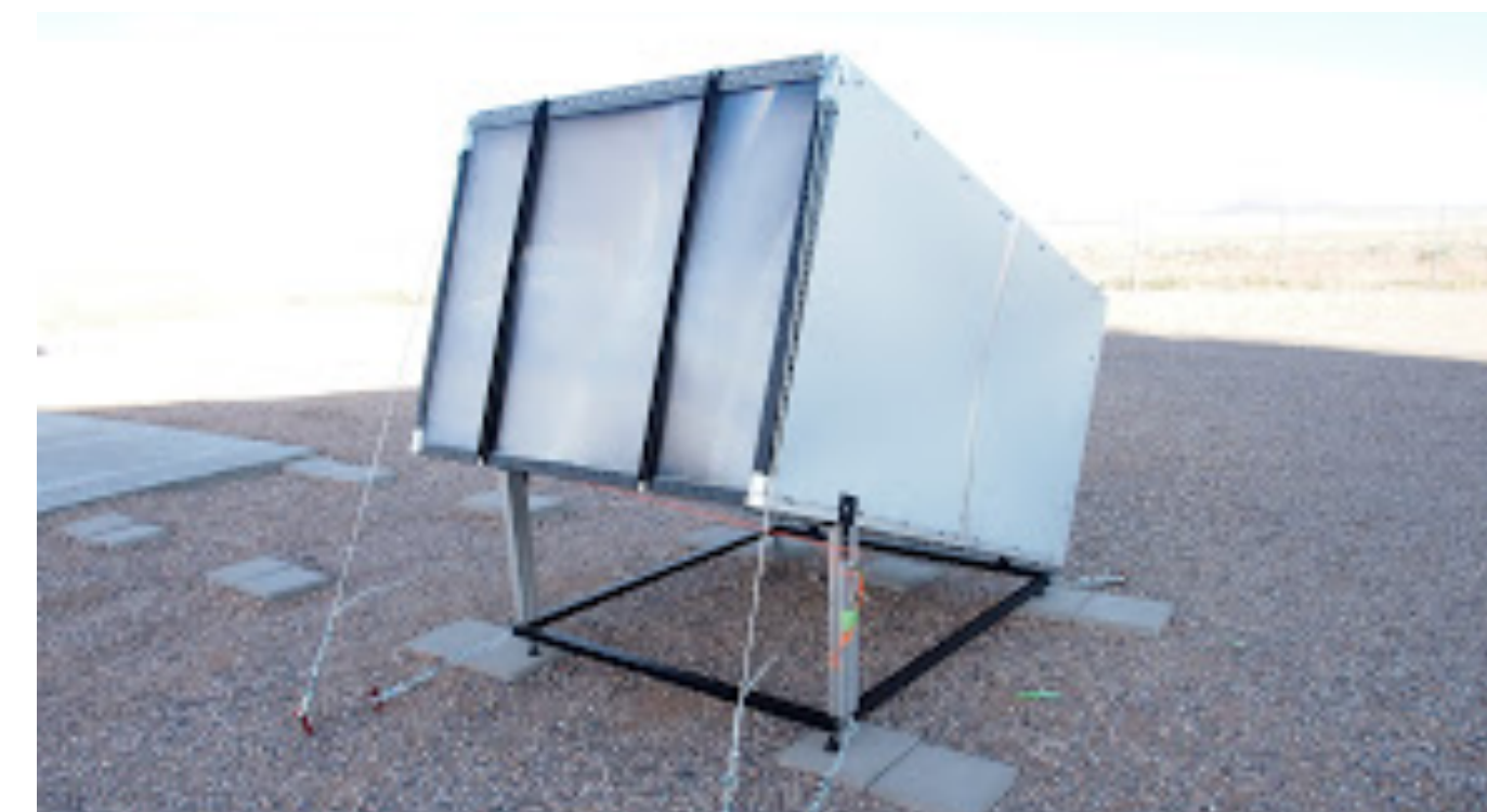
Fig1. Exterior of CRAFFT detector which consists of Fresnel lens, UV trans. Filter, 8 inc. PMT, FADC.
