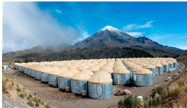
Figure 1 The HAWC observatory and Pico de Orizaba. Three hundred WCDs arranged in a regular array can be utilized as a hodoscope to observe nearly horizontal muons.
