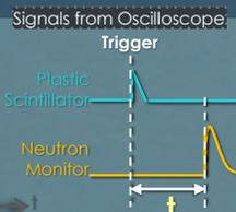
Experimental setup, with charged particle detectors (scintillator and Si PIN array as prototype satellite detector components) placed on top of the Princess Srinthorn Neutron Monitor (PSNM) at the summit of Doi Inthanon, Thailand. The signal from charged particle detector was used as a **trigger** to collect the waveform of the signal from the neutron monitor by oscilloscope. The trigger signal was set to be detected at  $0.5$  ms of total  $6$  ms time window of the oscilloscope.
