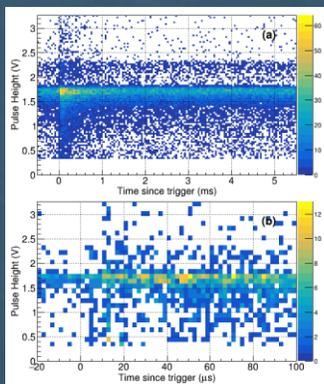
The distribution of pulse height and time relative to a charged particle trigger for each pulse in PSNM Tube 1 is shown in figure (left), (a) for all data ( $-0.5 \leq t < 5.5$  ms) and (b) for  $-20 \leq t < 100$   $\mu$ s.
