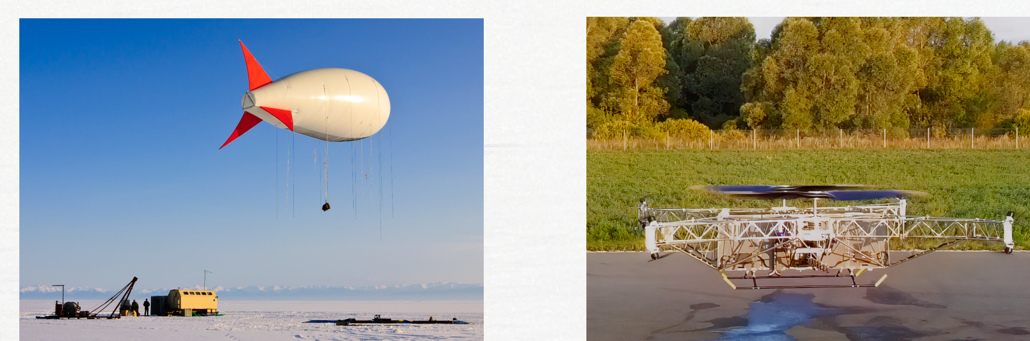
Fig. 3: The SPHERE-2 lifted by a balloon in March 2013 and an example of a heavy agricultural drone proposed as a carrier for the SPHERE-3 (Braeron ID-400A)
