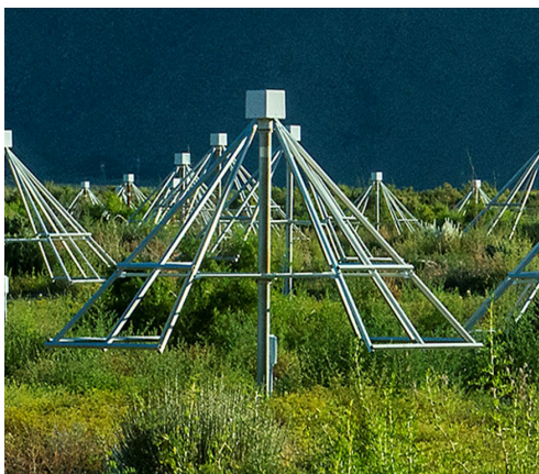
Figure 1: OVRO-LWA antennas (Photo: Gordon Wiltsie). The Owens Valley Radio Observatory lies between two mountain ranges in the sparsely populated region of Eastern California. The OVRO-LWA antennas' bandpass will be Galactic-noise-dominated from 12-85 MHz.
